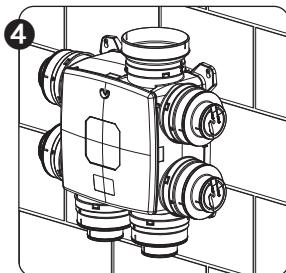
Put the number of desired sealing caps and/or reductions on the ventilation system and cut them open at the desired diameter. ( $\varnothing 80 \text{ mm} / \varnothing 125 \text{ mm}$ ). Close off the other extraction points on the unit with sealing caps.
