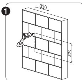
Put the mounting base of the Cbase® against the wall and transfer the position of the screw holes onto the wall with a pencil (wall has to have a minimal mass of 100 Kg/m<sup>2</sup> to avoid noise transference).
