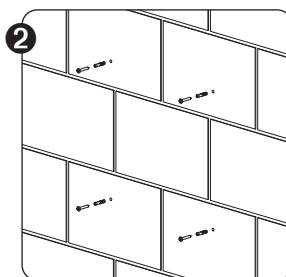
Mount wall plugs and screws (suitable for the type of surface) to the wall. Make sure that the heads of the screws stick out ± 7 mm.
