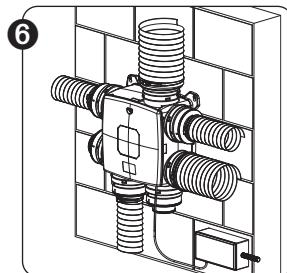
Unscrew the lid of the ventilation box. Make sure that the power is turned off! Connect the power cable and the cable for the three position switch according to the electrical wiring scheme (section 6.1).
