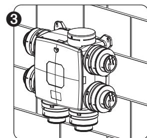
Hook the ventilation system over the 4 screws. Make sure that the exhaust of the unit is placed toward the roof/wall outlet.
