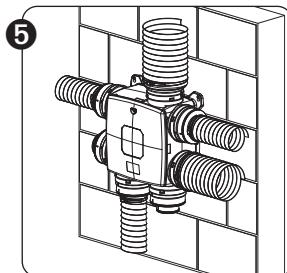
Connect the ventilation ducts to the reductions by means of fixing straps.
